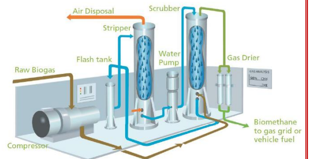
Fig. 4 : Water Scrubber System
