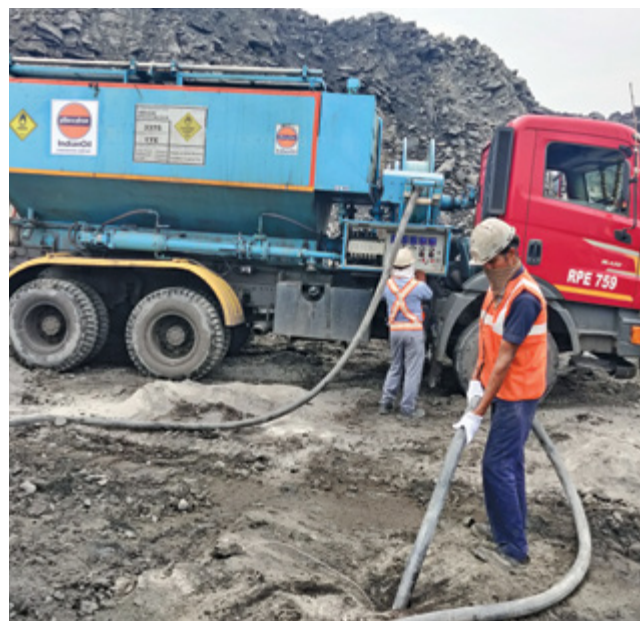
Charging of bulk explosive at a mine site
