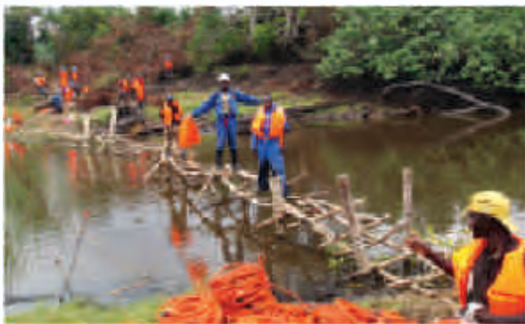
Laying a seismic cable across a river at Gabon
