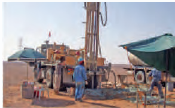
Truck mounted drilling rig for uphole measurement at Libya
