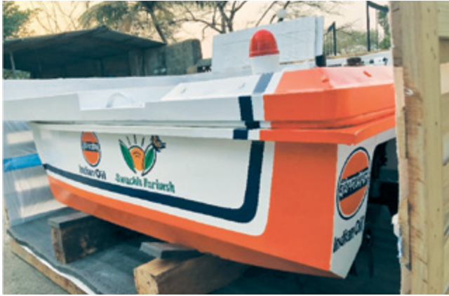
Remote-operated water drone (Floater Boat)
