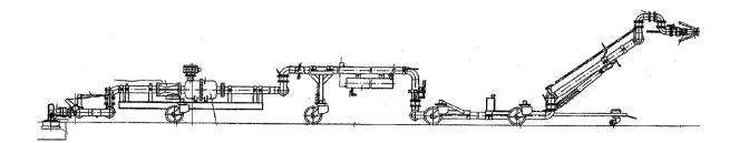
The pantograph is used to refuel aircraft from a Hydrant Refuelling System. Pantograph Refuelling is a maintenance-free operation which involves a stainless pipes that stretch to connect to the aircraft refuelling point. The pantograph shall be used to refuel Jet A1 to aircrafts. The major components of the pantograph are the following:
