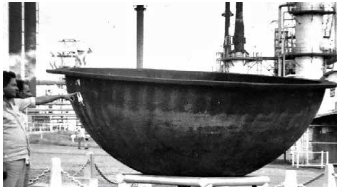
'The Still' precursor of petroleum refining, used to treat crude oil around 1890s, exhibited inside Digboi Refinery - Huge cast iron cauldron on 9 feet diameter
