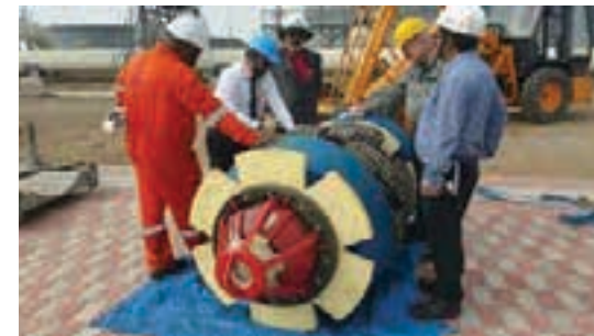
Circumferential MFL tools used to detect axially oriented metal loss and lone seam crack like anomalies
