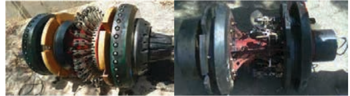
Caliper tools used to detect bore reduction and other geometry related anomalies
