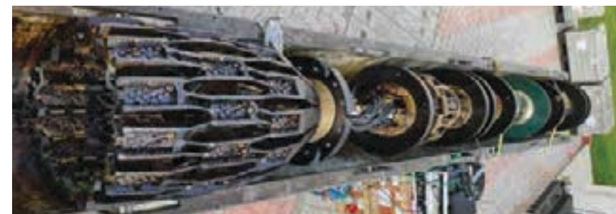
Circumferential MFL tools used to detect axially oriented metal loss and lone seam crack like anomalies
