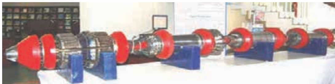
The first generation smart pig - 12" IPIG tool developed by IOCL R&D
