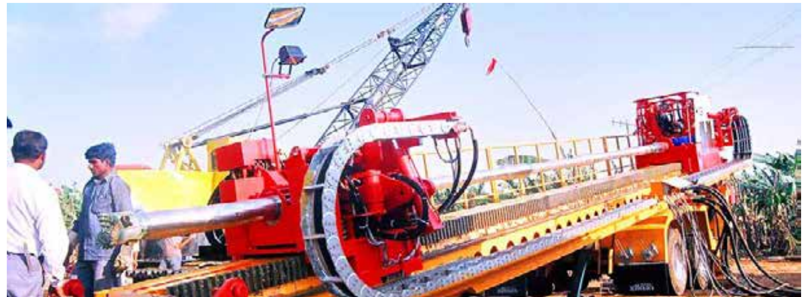
Horizontal Directional Drilling (HDD) Rig
