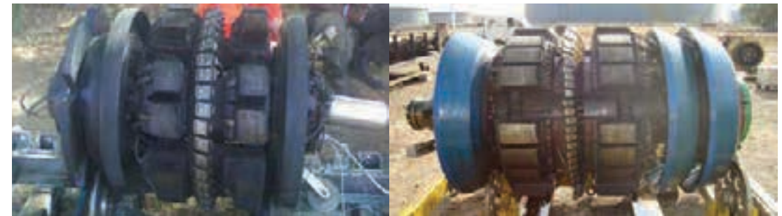
Axial MFL tools used to detect metal loss anomalies in pipeline
