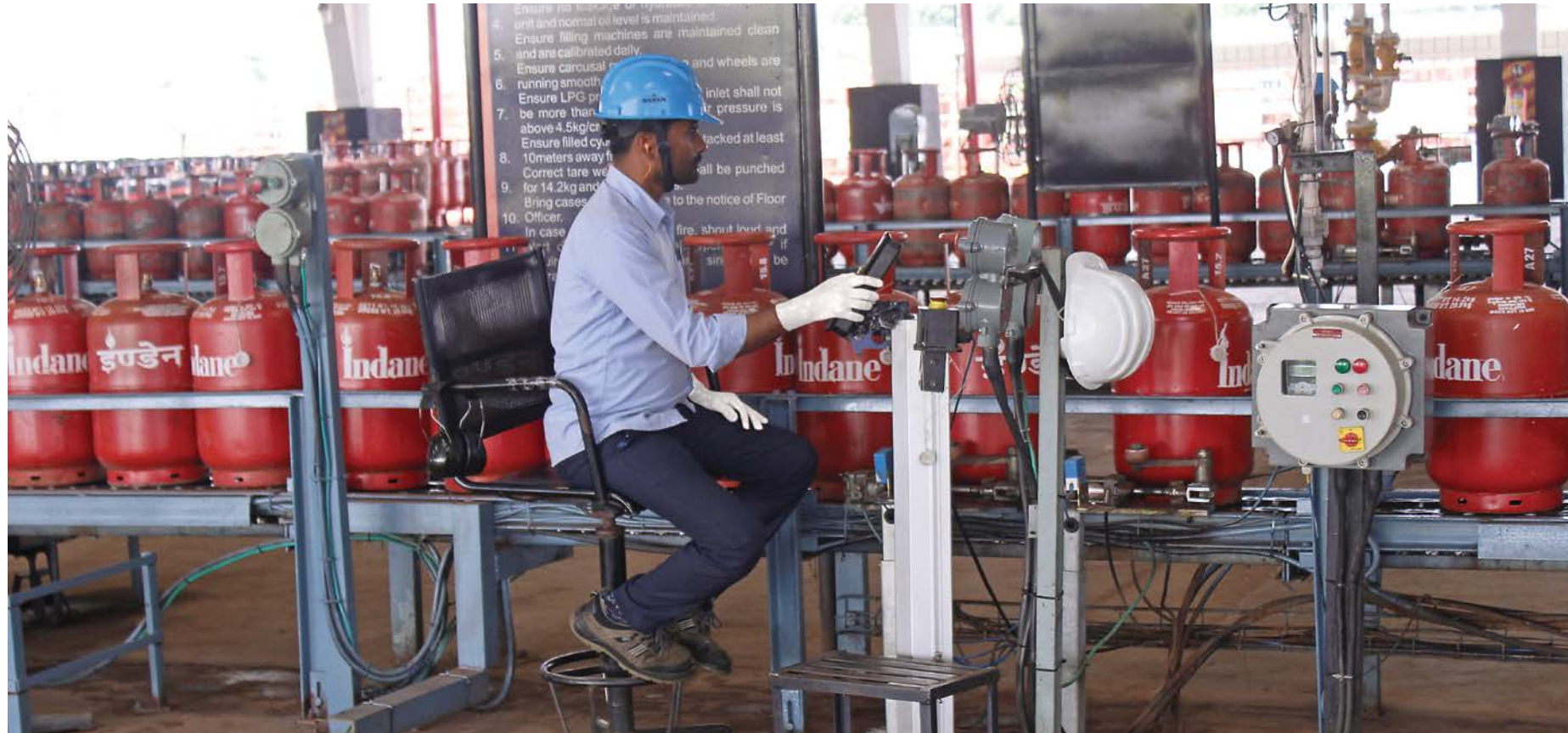
Punching of tare weight of LPG cylinders at the Mysore bottling plant.
