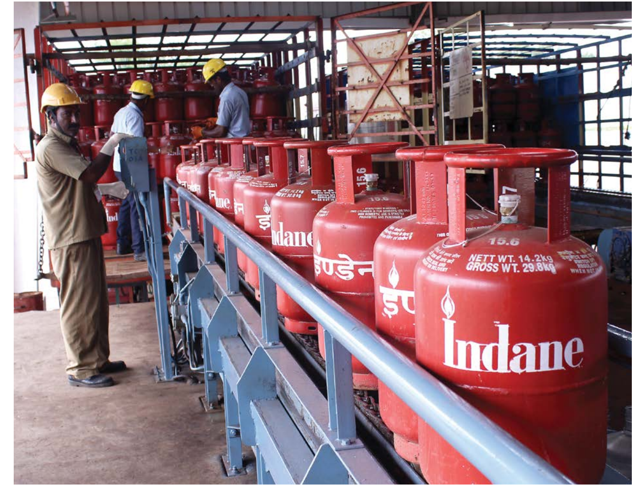
Unloading of empty cylinders from Packed LPG Trucks at the unloading shed of the Mysore bottling plant.
