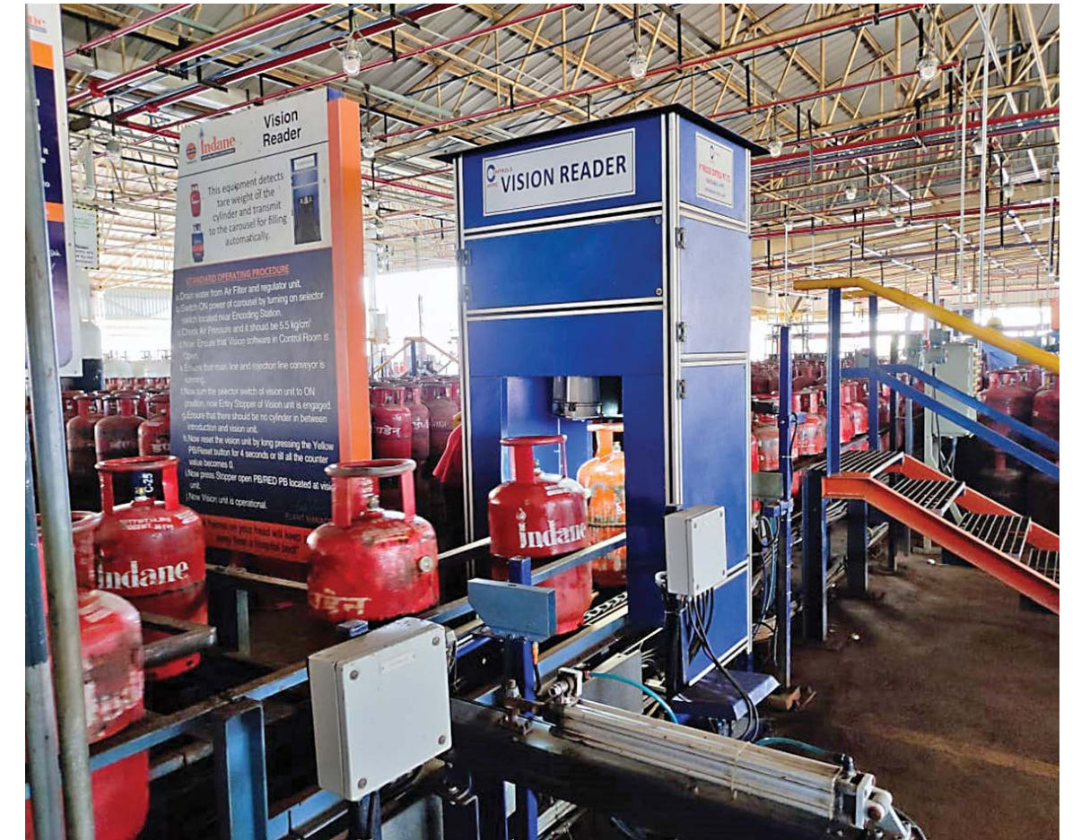
Vision Reader Unit for automatic capture of cylinder tare weight at the Salem bottling plant.
