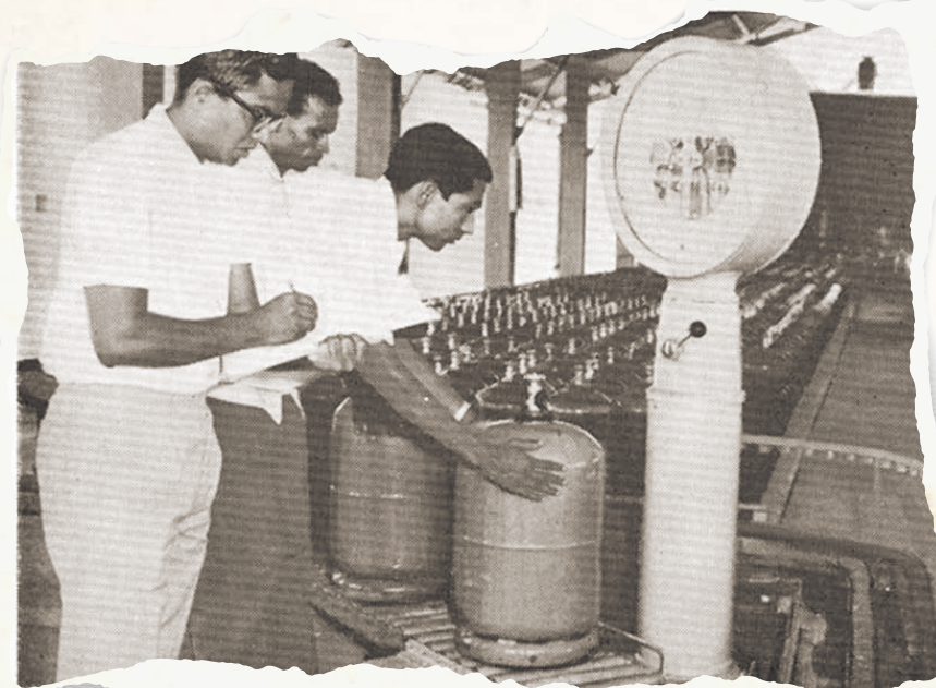
Personnel check accuracy of cylinder weight at the LPG bottling unit of Gujarat Refinery in 1968.
