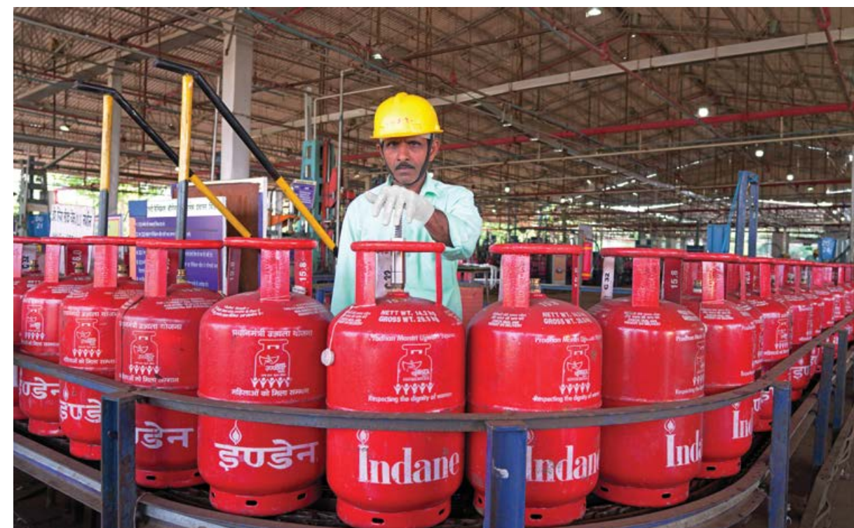
Checking and insertion of O-Ring in the SC valves of cylinders at the Bhopal bottling plant.
