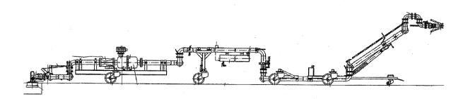
The pantograph is used to refuel aircraft from a Hydrant Refuelling System. Pantograph Refuelling is a maintenance-free operation which involves a stainless pipes that stretch to connect to the aircraft refuelling point. The pantograph shall be used to refuel Jet A1 to aircrafts. The major components of the pantograph are the following:
