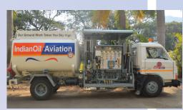
Currently, batches of 11 KL & 16 KL refuellers are in final stages of manufacturing.
