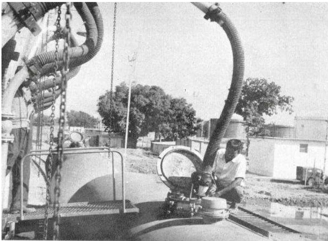
*Tank wagon filling at the loading racks at the Barauni Refinery.*
