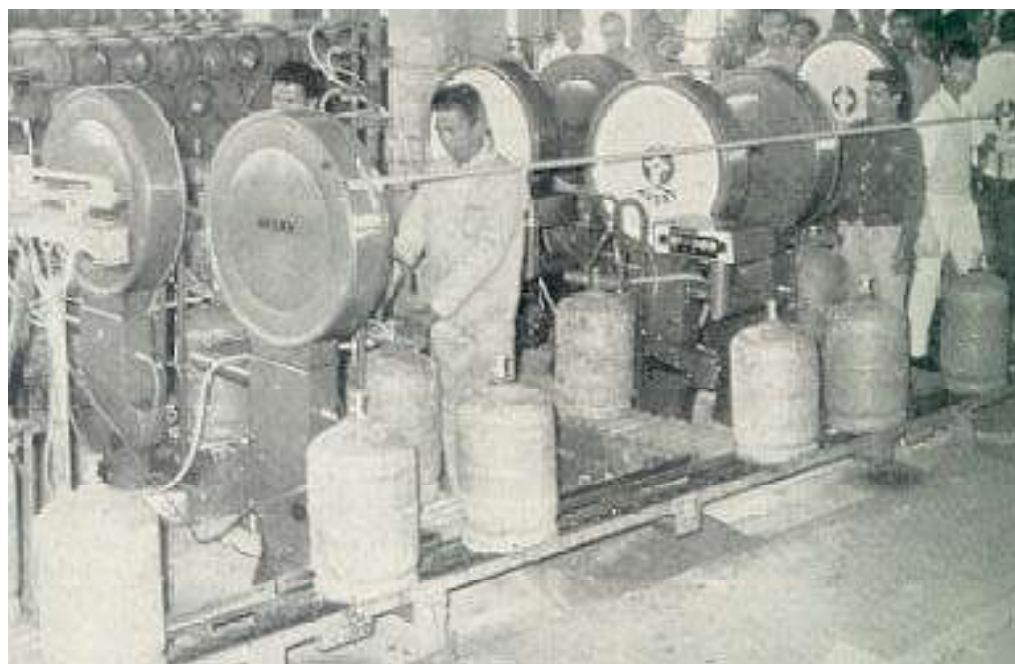
Filling of Liquefied Petroleum Gas cylinders by automatic bottling machines at the Gujarat Refinery
