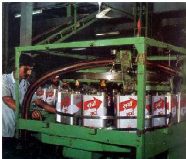
*Close supervision and automatic filling machines ensure quality and quantity in lubricant tins*
