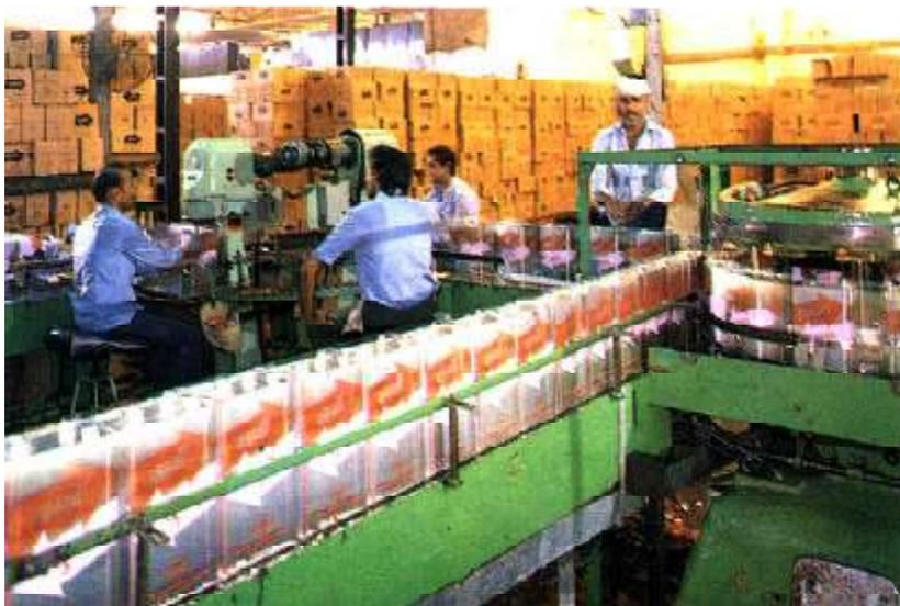
*Closed supervision and automatic filling machines ensure quality and quantity in lubricant tins.*
