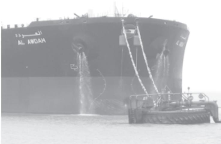
*Single Point Mooring off Vadinar coast in the Gulf of Kutch, the discharge point for Very Large Crude Carriers bringing in imported crude oil for onward movement to Koyali, Mathura and Panipat refineries by pipelines.*
