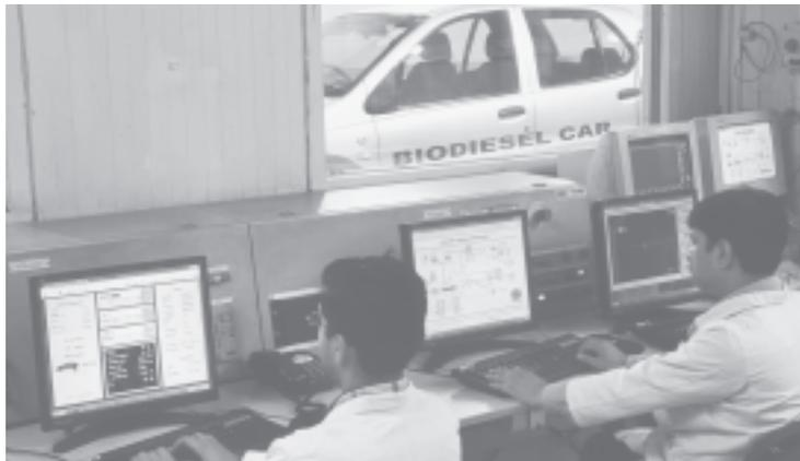
*IndianOil scientists conducting test runs on various blends of Bio-diesel with diesel in the climatic chamber of the R&D Centre as part of commercialisation efforts in alternative fuels.*
